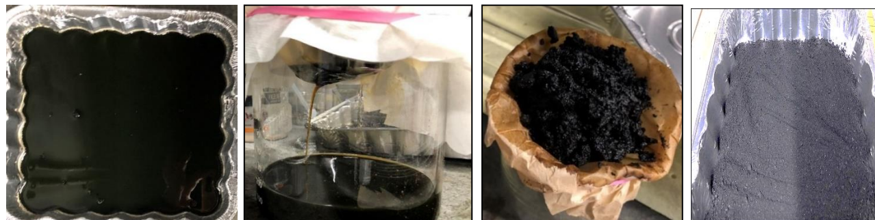
Figure XX: Toluene Bath Figure XXI: Initial Strain Figure XXII Final Strain Figure XXIII: Dried
