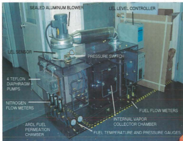
Figure 3: Complete Permeation Set-up
